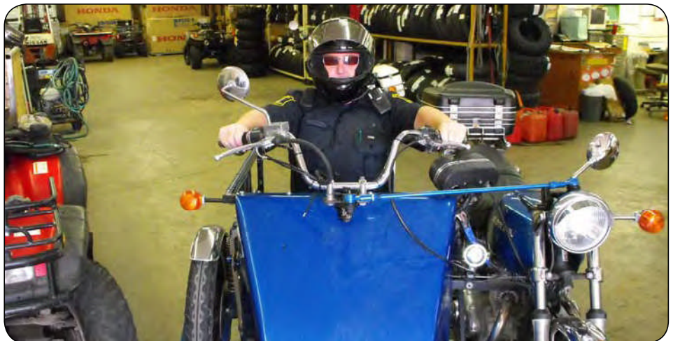
Front view of the adapted Honda with wheelchair sidecar.
